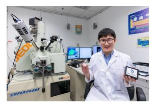
Image 1. Dr Yuqi QIAN and his lunar team will be using the Electron Probe Microanalyzer (EPMA), a highly advanced analytical tool located in HKU Department of Earth Sciences, to study the chemical composition of the lunar sample. This tool is capable of providing accurate and precise measurements of elements in the sample, making it a valuable asset for the team's research.
